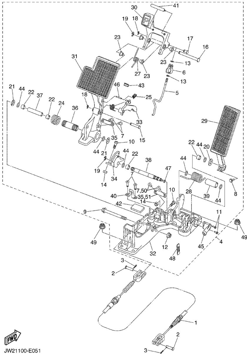
FIG. 5 PEDAL ASSEMBLY
